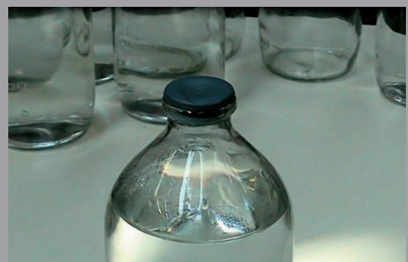
Sensors 4: Check of fill level and tightening of plastic cap.
